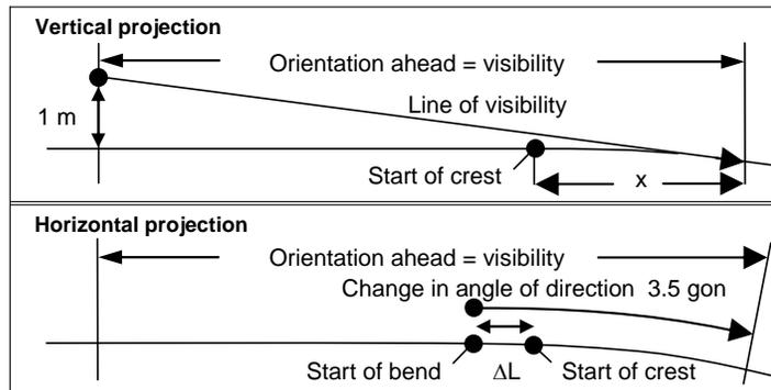
FIGURE 6 Model projection of a concealed start to a bend (4).
