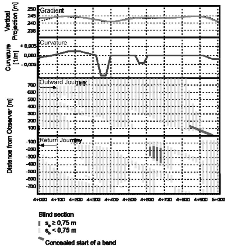
FIGURE 7 Blind section graph with a critical blind spot area and concealed start of a bend (6).
