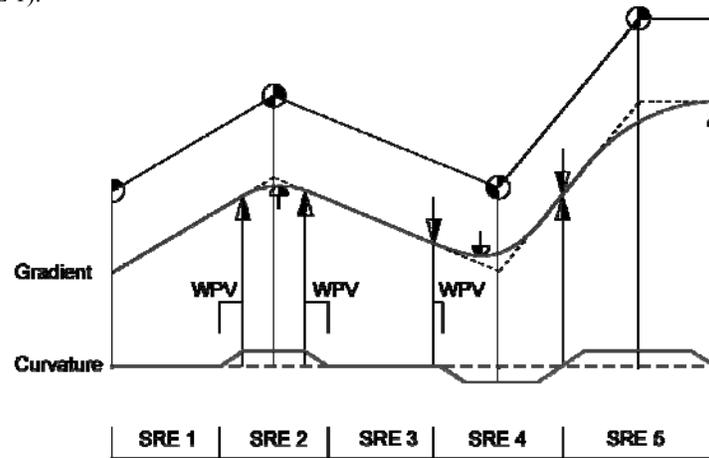
FIGURE 1 Standard sequence of three-dimensional elements (2).
