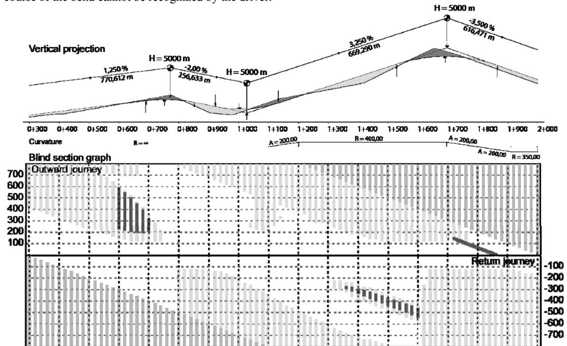
FIGURE 9 Blind section graph with critical blind spot area and concealed start of the bend (5).
