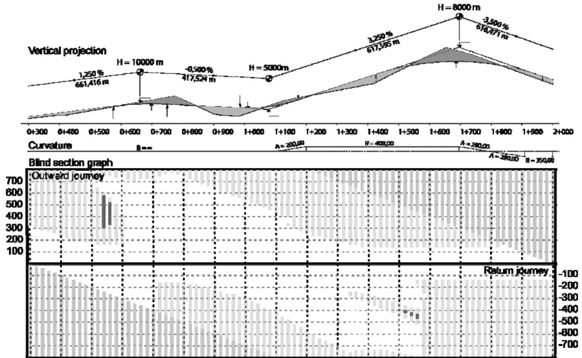
FIGURE 10 Blind section graph with critical blind spot area after the first redesigning stage (5).
