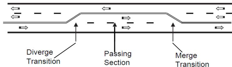
**FIGURE 2 Schematic example of three-lane alternate passing design. (3)**
