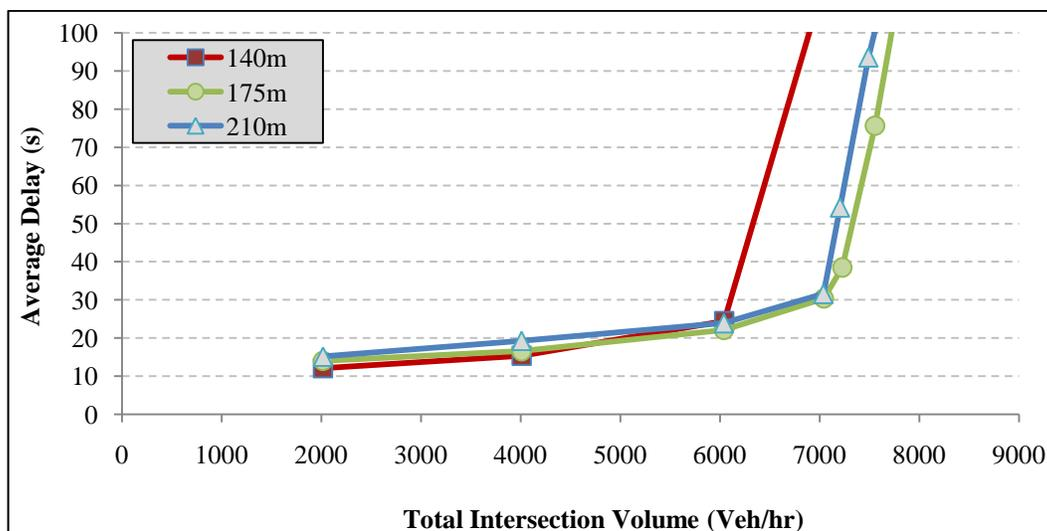
Figure 2 Delay Variation with Intersection Spacing Change for the Half USC Design
