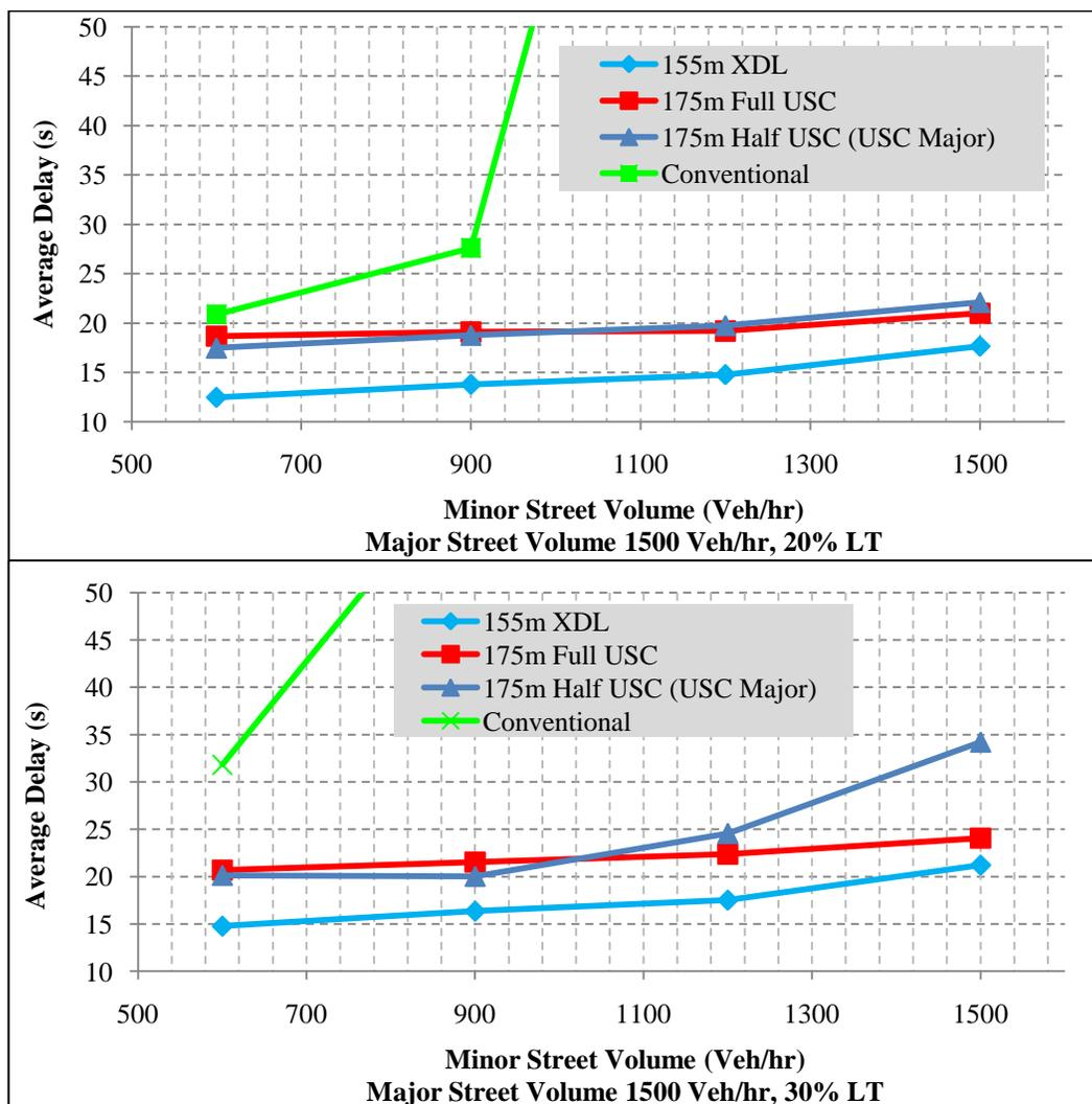
**Figure 8 Average Delays of The Analyzed Unconventional Intersections under Unbalanced Volume Scenarios**
