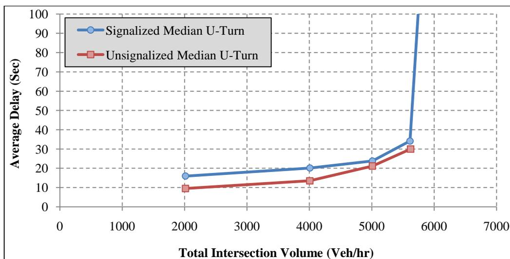
Figure 3 Delay Comparisons of Signalized and Unsignalized U-turn Designs
