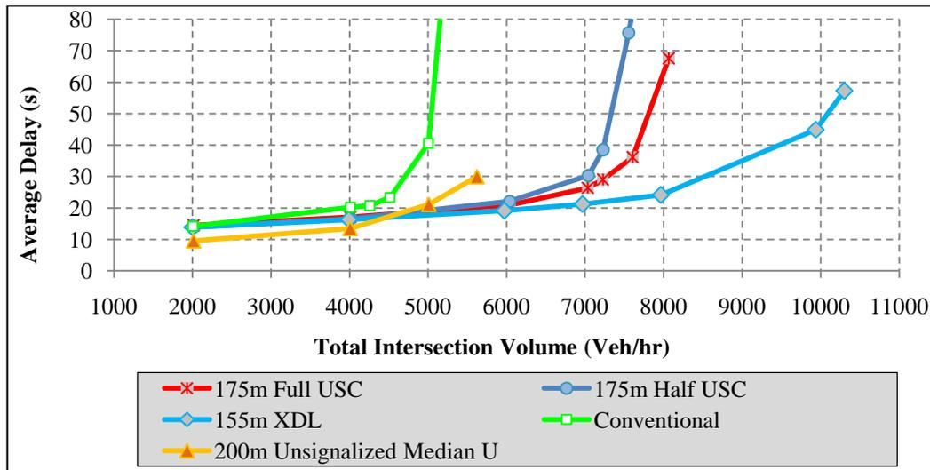
**Figure 4 Average Delays for the Analyzed Intersections Under Balanced Volumes (20% LT)**
