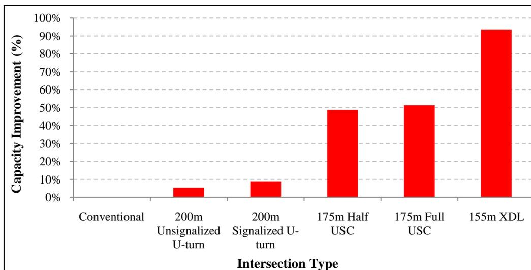
**Figure 5 Capacity Improvements of the Unconventional Intersections in Comparison to the Conventional Intersection**
