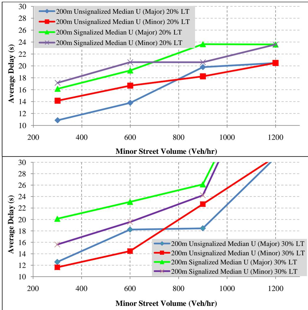
**Figure 7 Average Delays for Median U-turn Intersections under an Unbalanced Volume Scenario, Major Street Volume = 1200 Veh/hr**
