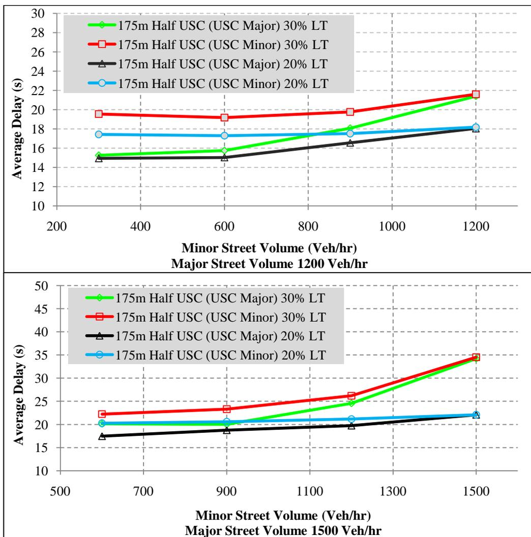
Figure 6 Average Delays for the Half USC Intersections under Unbalanced Volumes
