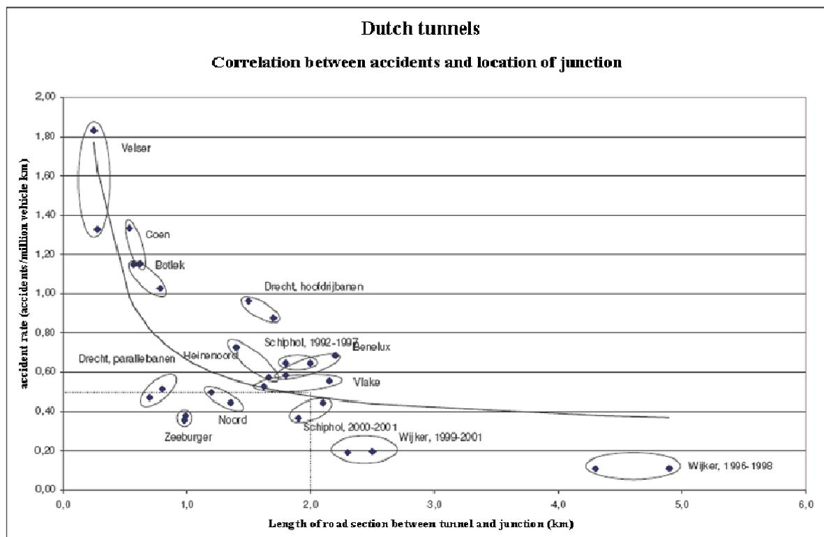
**FIGURE 3 Relation between accident rates and the distance between a tunnel and the nearest junction**
