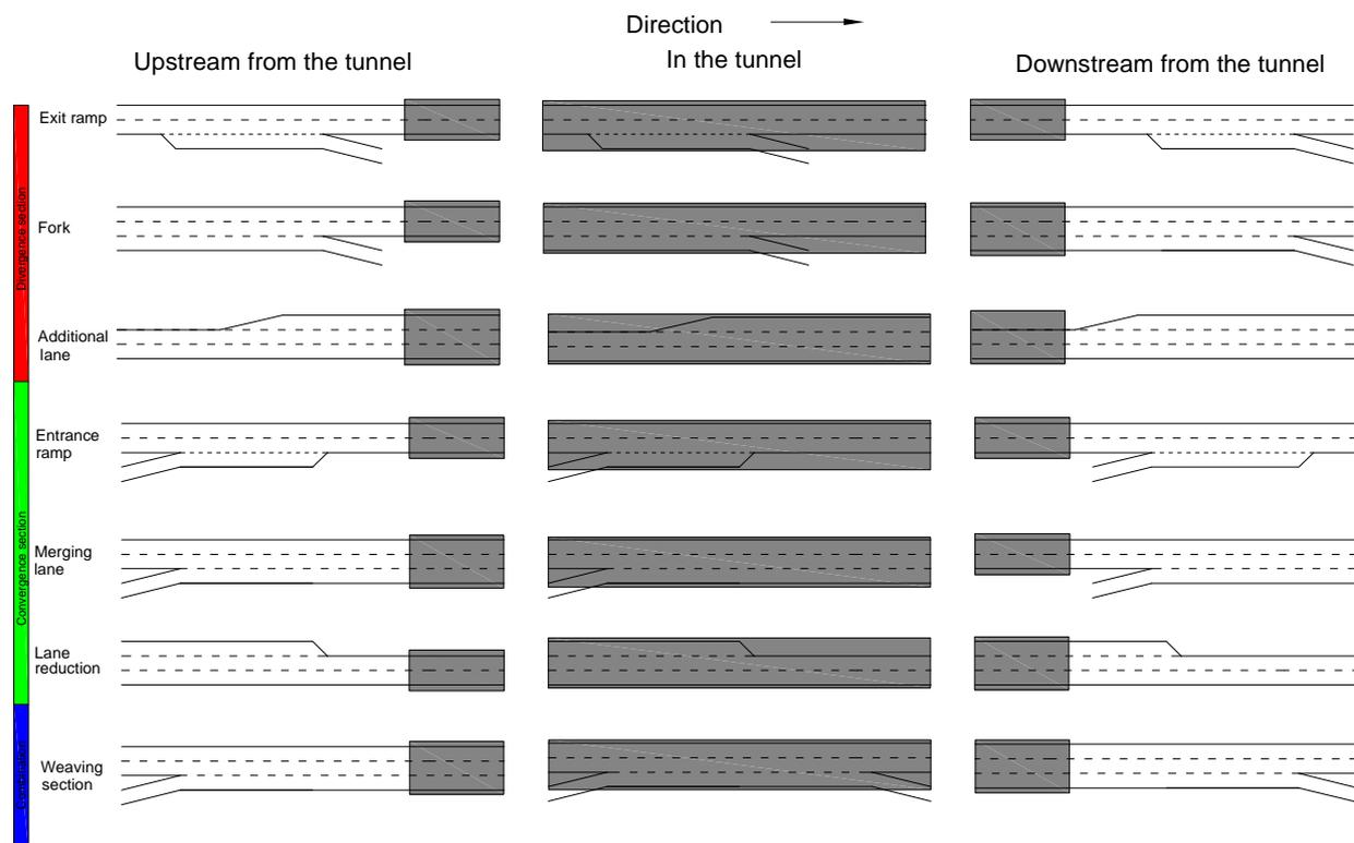
**FIGURE 2 Possible combinations of convergence and divergence sections with a tunnel**
