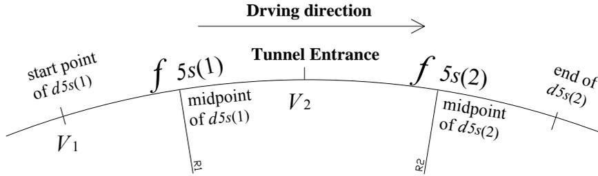
FIGURE 1 Alignment index at tunnel entrance.
