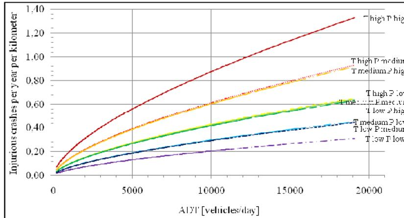
**FIGURE 3 Abacus of accident prediction models on roads with undivided roadways where  $L_a=10.50$  m and  $V=70$  Km/h.**
