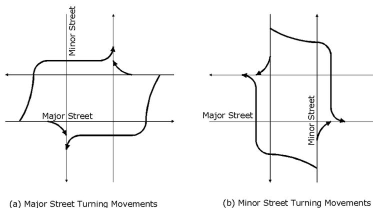
**Figure 1 Vehicle Movement at a Full Continuous-flow Intersection**
