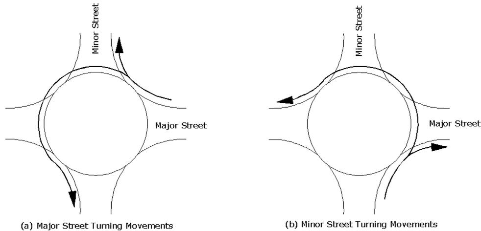
**Figure 5 Roundabout Turning Movements - Example**
