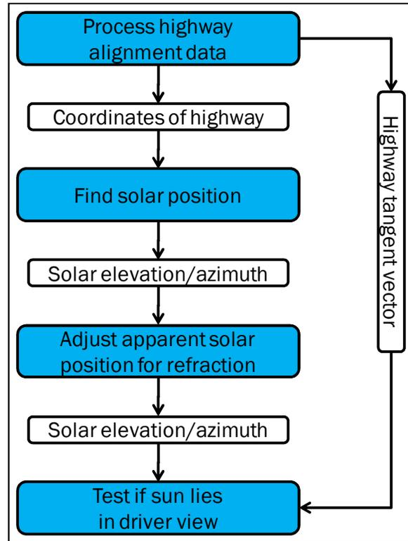
Figure 1 – Sun glare algorithm flow chart
