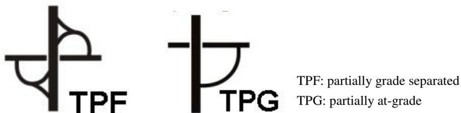
**FIGURE 2 Selected junction types according to the new guidelines for the design of rural roads (RAL) currently being developed (FGSV, 2007)**
