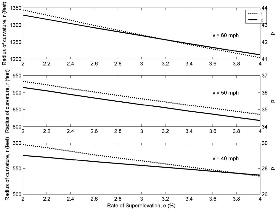
Figure 5. Effects of Varying Speeds on Radius of Curvature, Superelevation, and P.
