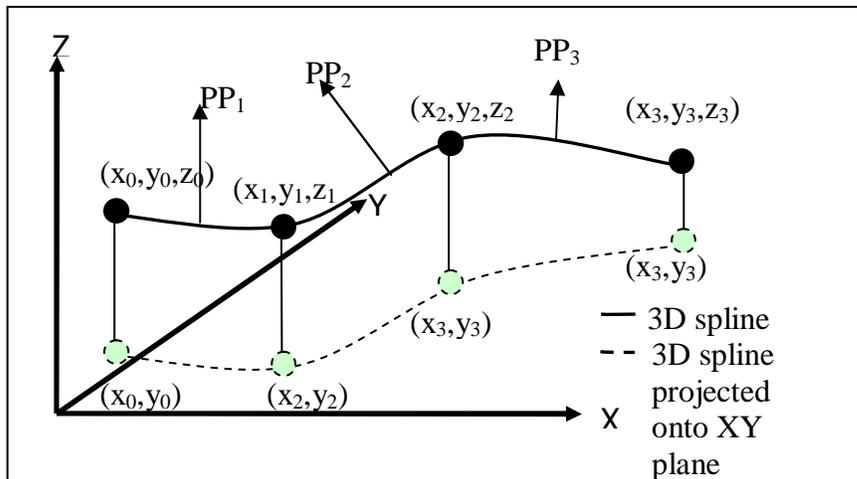
**Figure 2:** A typical 3D spline. Here 3D spline has three piecewise polynomials  $PP_1, PP_2, PP_3$  with four knots.
