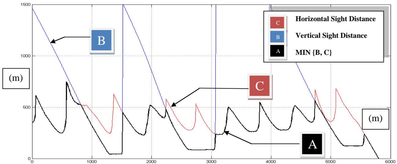
**Figure 8. Horizontal and Vertical Sight Distance**
