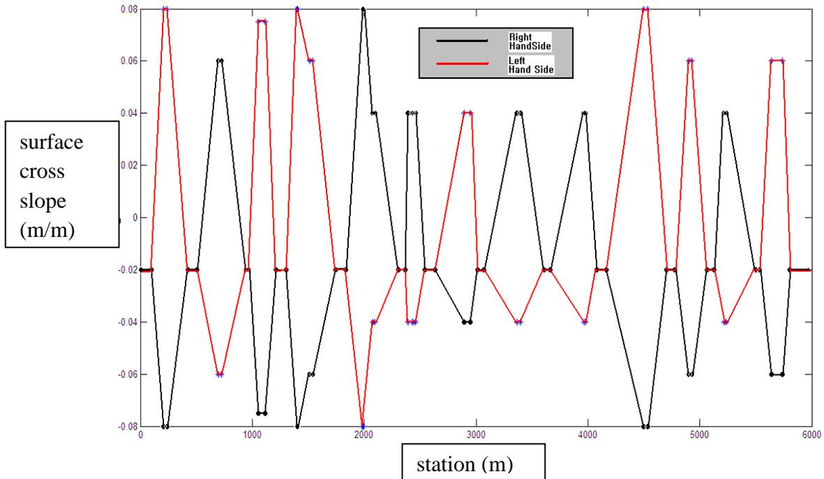
(a) Surface Cross Slopes on Example Alignment
