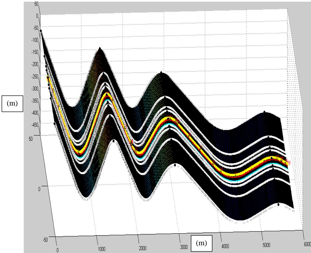
**Figure 7. Road Shape for Vertical Sight Distance**
