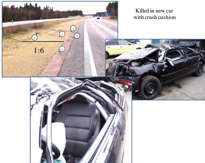
**Figure 6** - Typical severe wide 1:6-sloped motorway median accident from E4 Jönköping county
