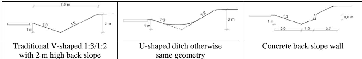
**Figure 12** – Full-scale test designs
