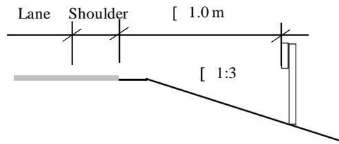
**Figure 3** - Basic principles of the slope guard-rail.
