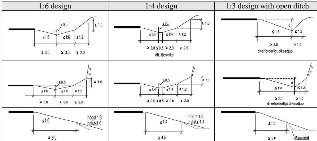
**Figure 2** – VU94 roadside design alternatives
