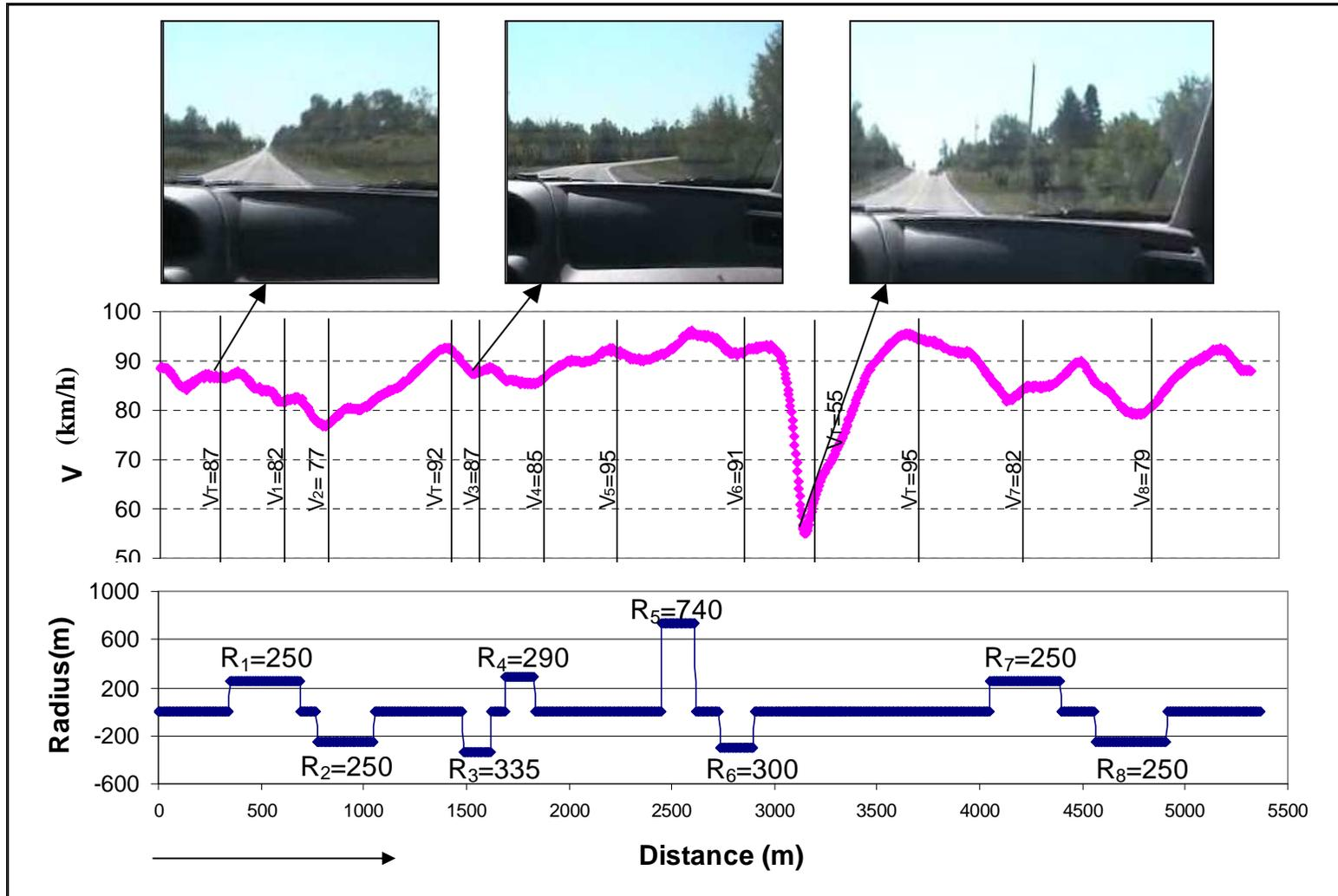
Figure 6. Alignment, Speed and Driver's View for Part of RR3
