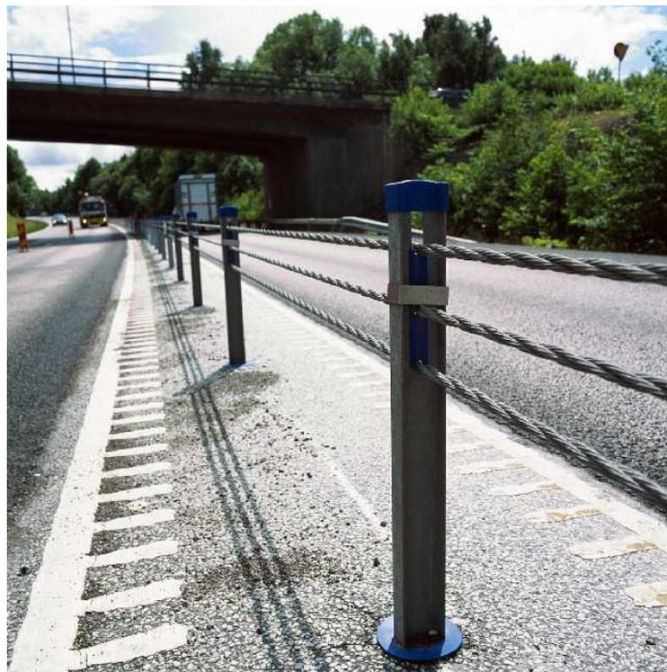
Figure 1. Movable cable barrier on a 2+1 roadway in Sweden.
