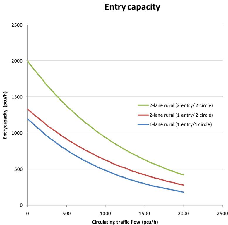
FIGURE 4. Entry capacity at 1- and 2-lane roundabouts
