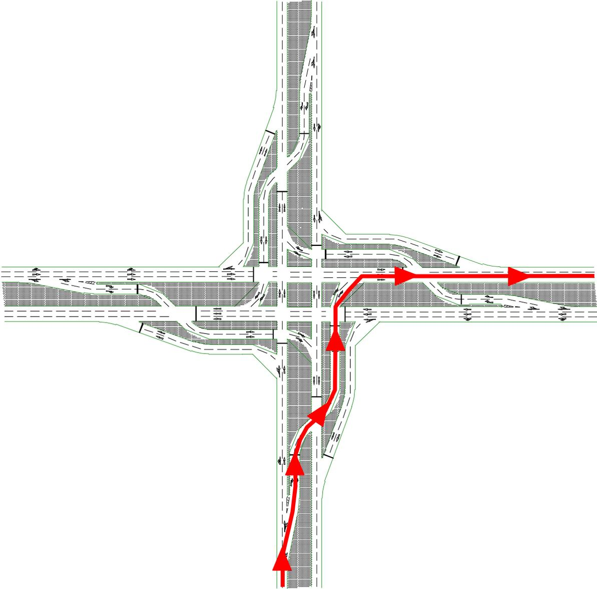
Figure 3 - 4-arm Displaced Right Turn intersection (DTR)
