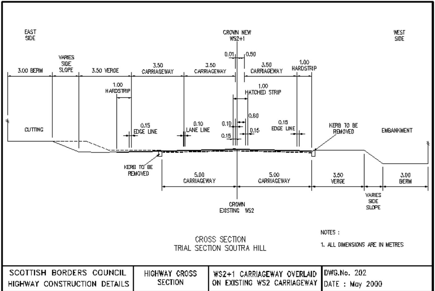
Figure 2 - WS2+1 cross section at A68 Soutra Hill Scotland.
