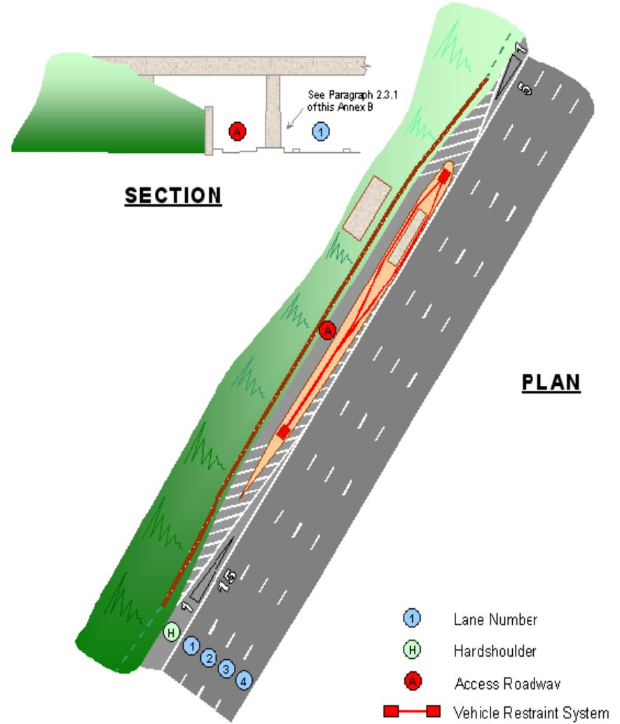
**Figure 9 - Layouts for maintaining emergency access at a discontinuity of the hard shoulder at an obstruction or structure (Taken from TD27/05 Cross Sections & Headroom's)**
