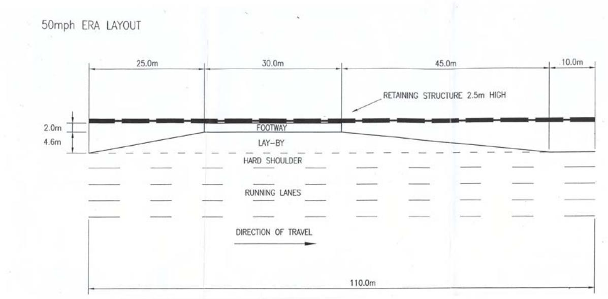
Figure 5 - Layout for Emergency Rest Area as proposed for the M42 ATM project
