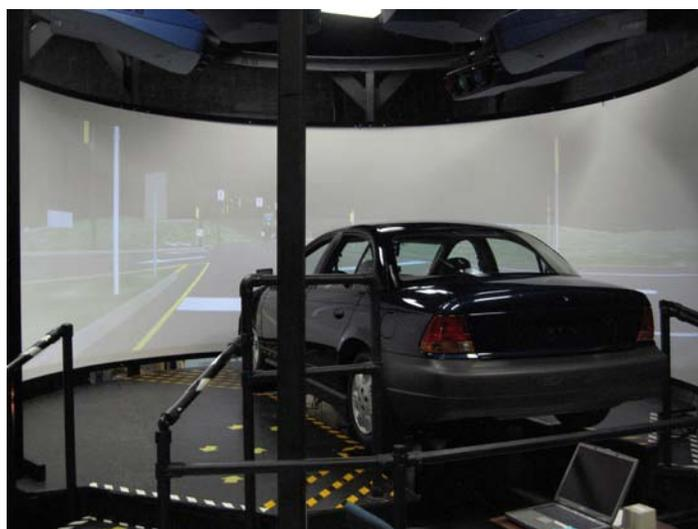
The Federal Highway Administration can estimate human capabilities and limitations on various highway designs using this simulator at the agency's Turner-Fairbank Highway Research Center near Washington D.C.
