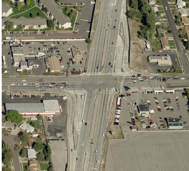
The displaced left-turn (DLT) intersection is located near Salt Lake City, Utah.
