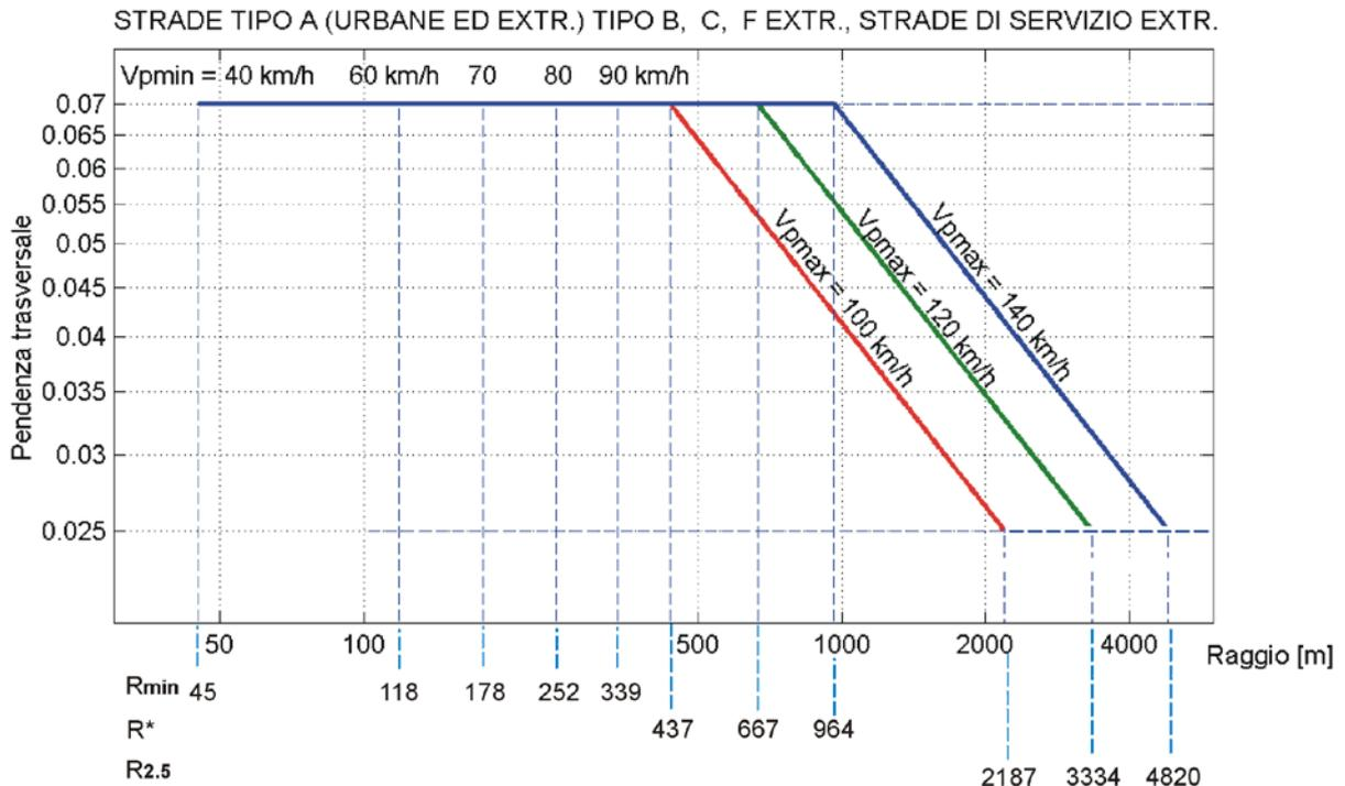
**Figure 6 Diagram to calculate cross fall and design speed vs. curve radius ( $V_p \equiv V_{design}$ )**
