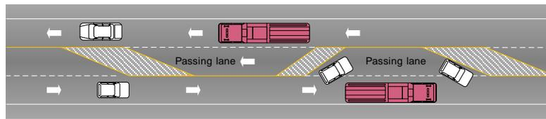
Figure 1 Graphical Representation of 2+1 roadway
