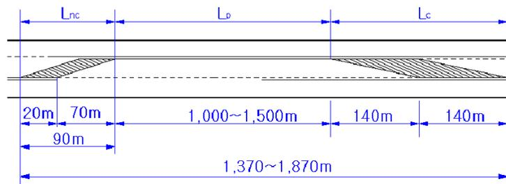
Figure 6 Configuration of the transition area for 2+1 roadway
