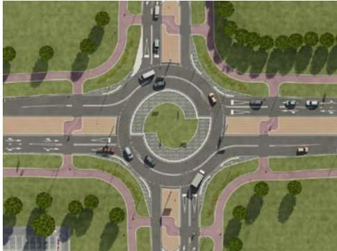
Figure 2: Turbo roundabout
